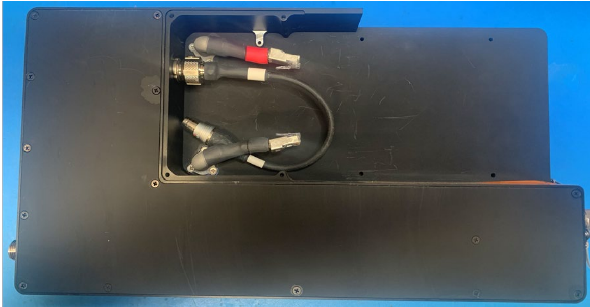
Figure 6 CORE with Network Encryptor Access Panel Removed
