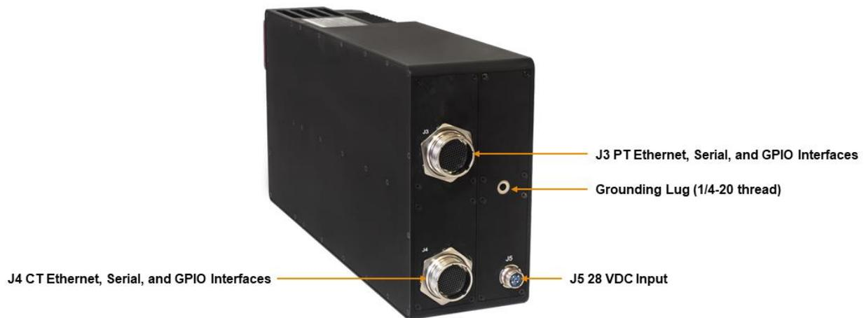
Figure 2: Rear view of CORE
