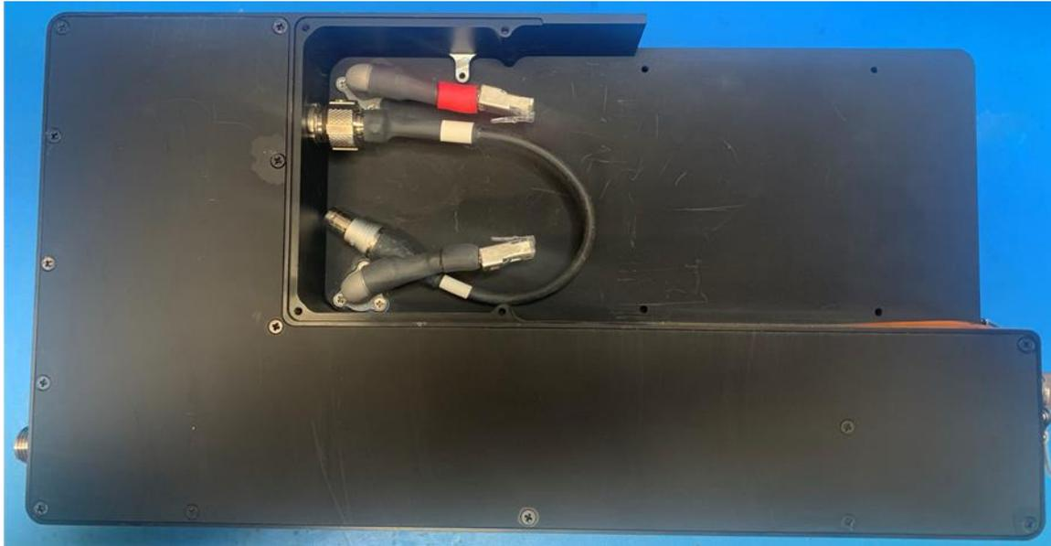
*Figure 6 CORE with Network Encryptor Access Panel Removed*
