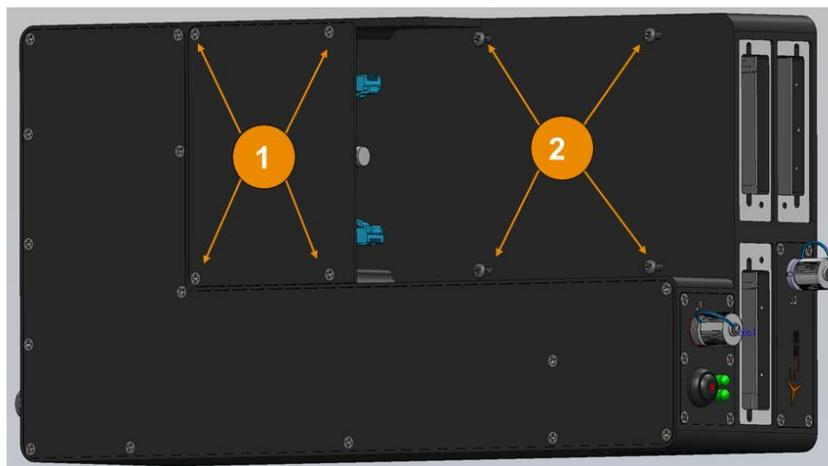
Figure 5 Diagram of Encryptor Mounting Screws on CORE
