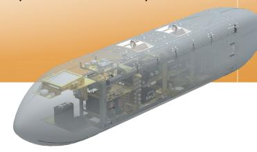
Fuse's KRAKEN 26 integrates the TENTaCLE architecture into an AgilePod® 26 airframe with a combination of SATCOM and LOS links.. The underwing pod approach brings a rapid-prototyping capability that moves faster than in-aircraft integration can deliver.
