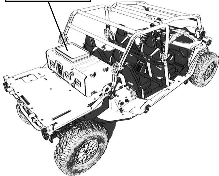
The KRAKEN UTV provides an excellent ground-based rapid-prototyping platform, capable of carrying modular payload racks, radios, and edge-compute equipment with ample mounting surfaces for antennas, sensors, and masts across the vehicle.
