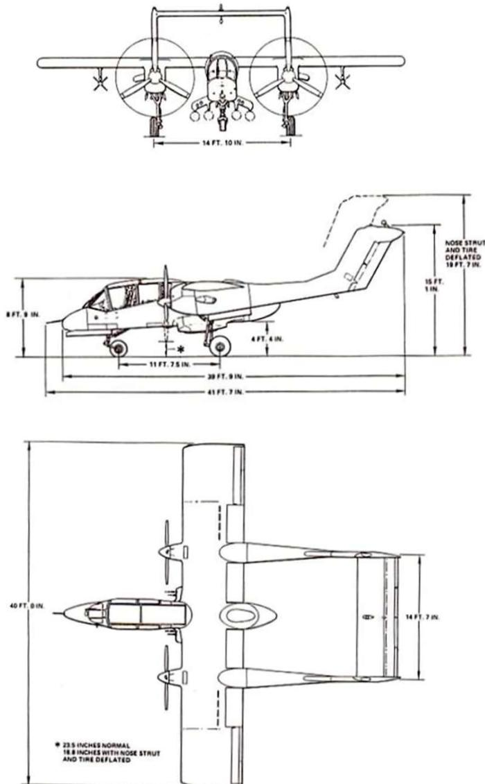
Fuse warfighter-focused design, engineering, development, and test includes a North American Rockwell OV-10 Bronco light twin turboprop aircraft with seven pod mounting pylons.
