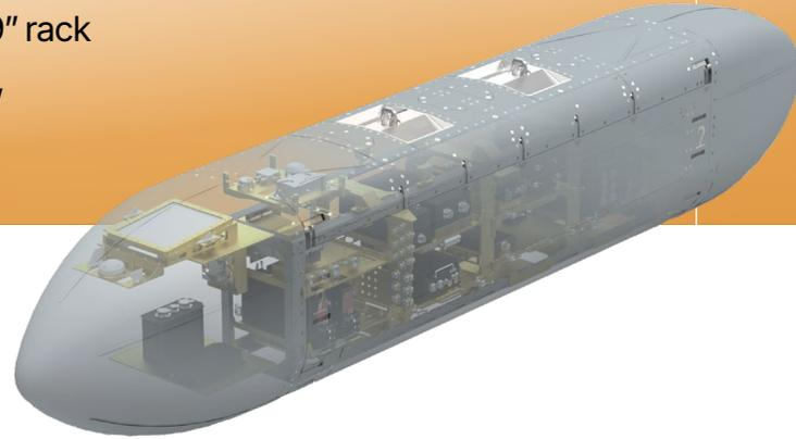
Fuse's KRAKEN 26 integrates the TENTaCLE architecture into an AgilePod® 26 airframe with a combination of SATCOM and LOS links. The underwing pod approach brings a rapid-prototyping capability that moves faster than in-aircraft integration can deliver.
